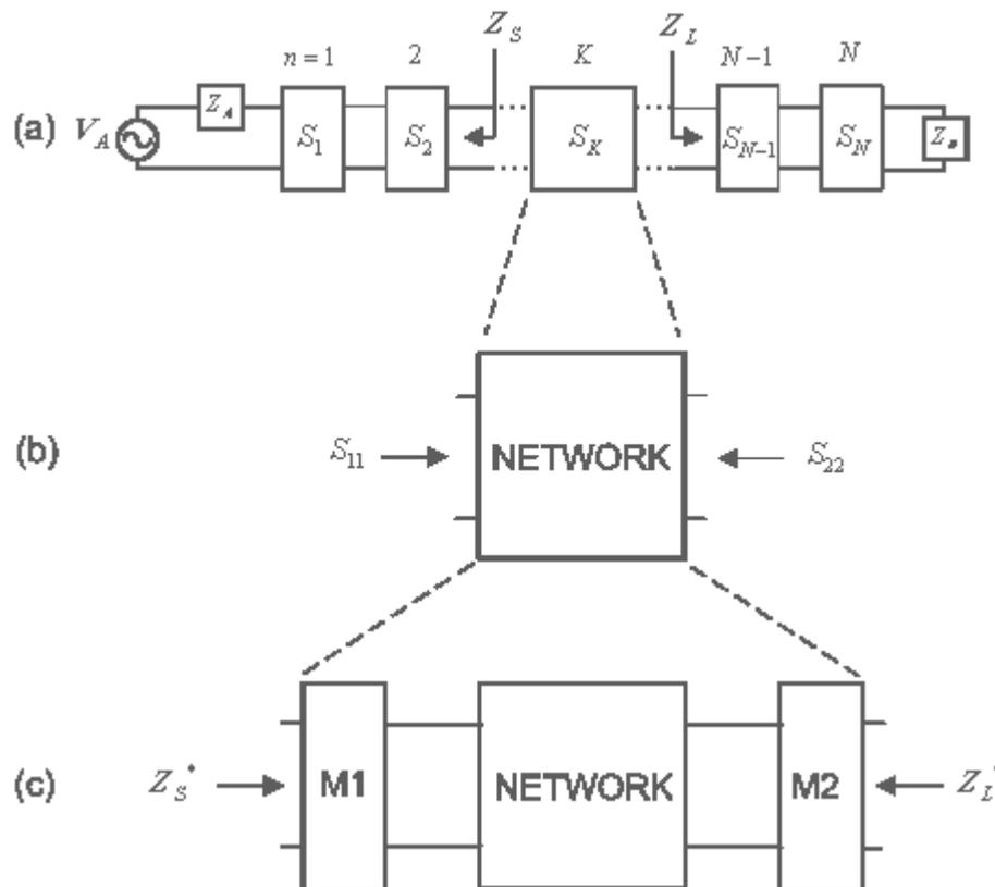
**Figure 2-1** A schematic showing two ways of substituting a 2-port network into a cascade: unmatched (a) and simultaneously conjugately matched (b)
