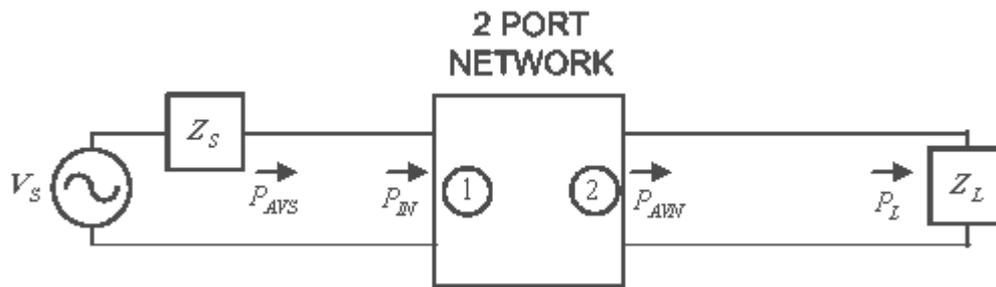
**Figure 1-2 The 2-port network connections showing the power definitions**
