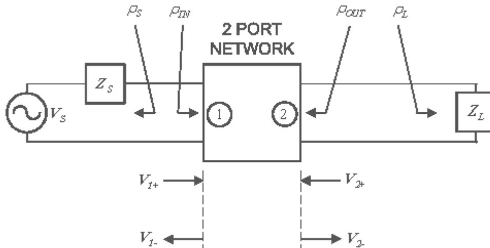
**Figure 1-1 Some general 2 port network connected to an arbitrary source and load**
