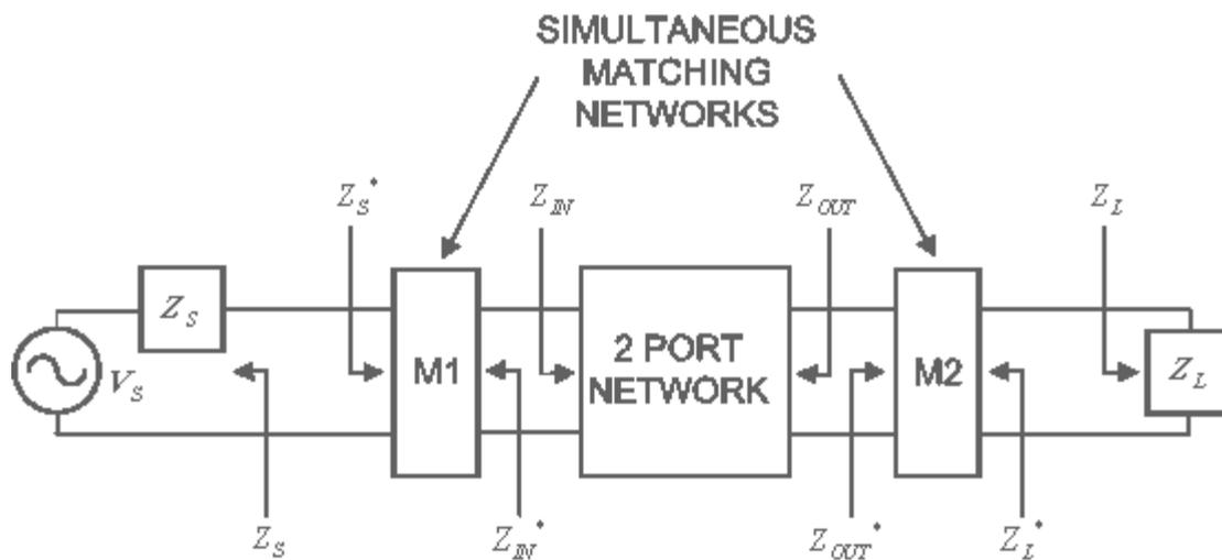
**Figure 2-2 A generic 2-port network that is simultaneously conjugately matched to a source and load**
