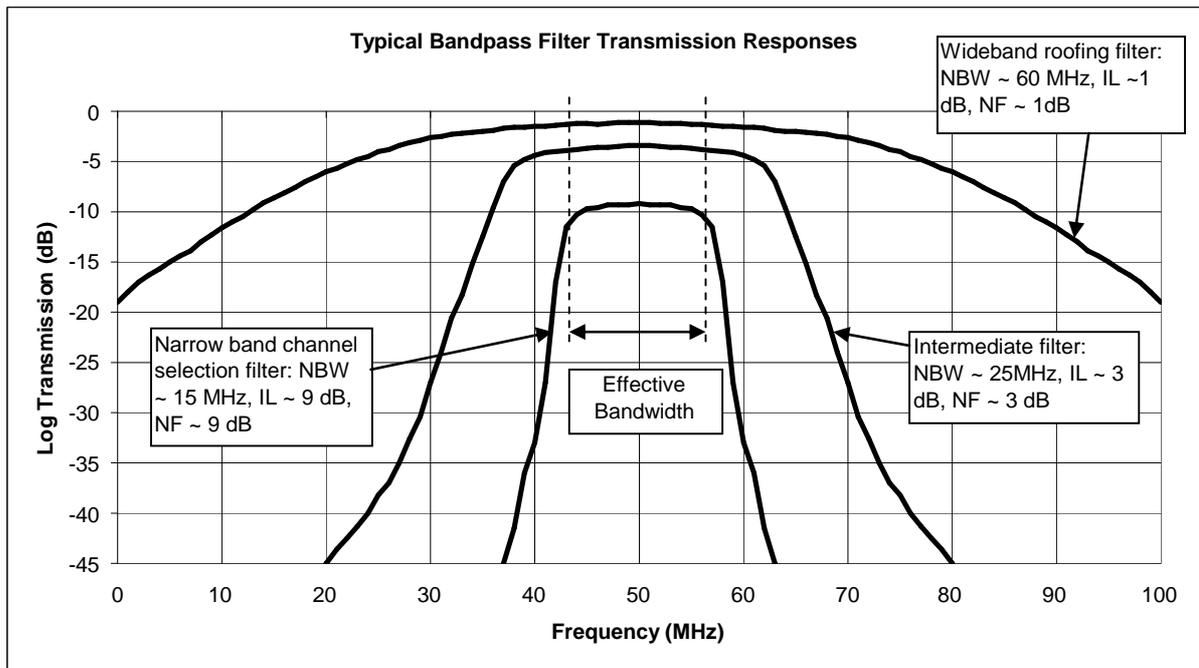
This analysis shows how the ultimate bandwidth achieved is determined by the last and narrowest filter that is encountered. Why then do we not simply put in a very narrow band filter right at the front of the cascade? There are several reasons:
