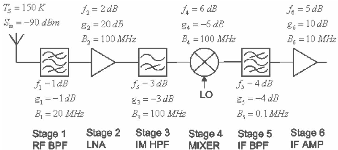
It comprises filters, amplifiers and a mixer. Each stage has a noise figure, gain and noise bandwidth:  $f_n$ ,  $g_n$  and  $B_n$  respectively. The subscript  $n$  represents the stage number, starting at 1. Lower case symbols are used for logarithmic (dB) quantities, and upper case symbols for their linear equivalents. So for example
