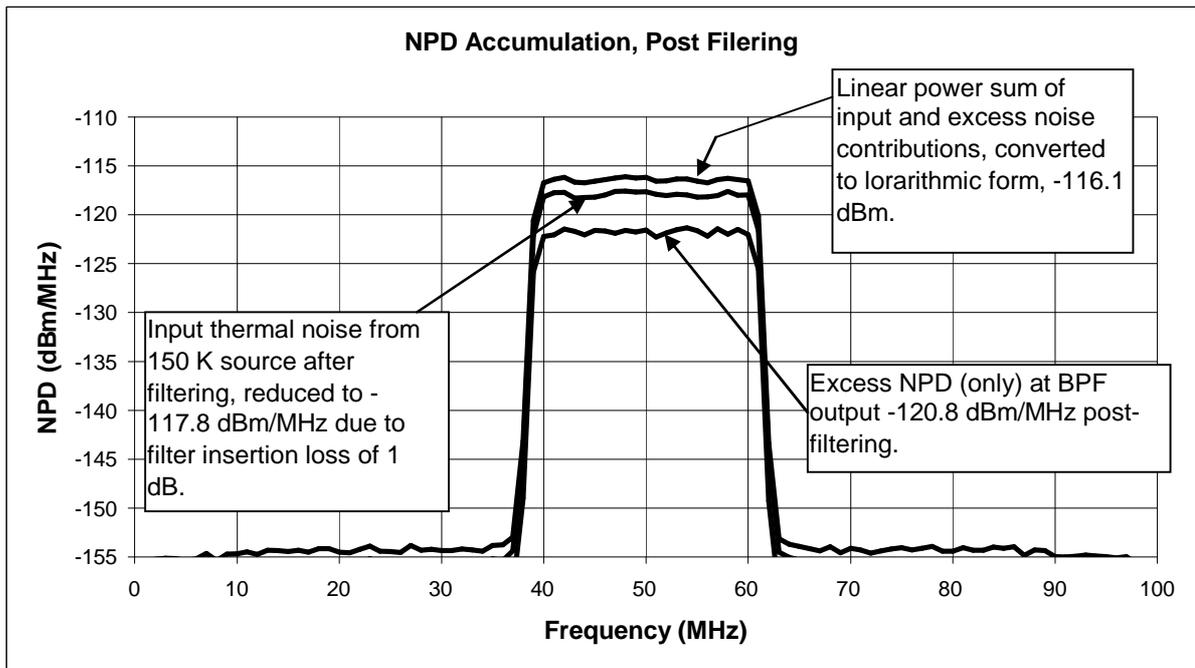
The same principles are applied to determine the NPD at later stages in the cascade.
