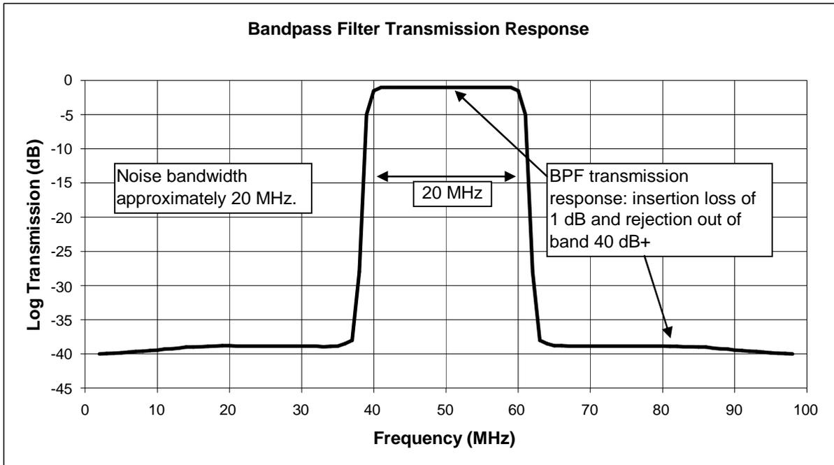
Supposing the noise temperature of the noise source at the input is at 150 K. There would then be two sources contributing to the noise measured at the output of the filter:
