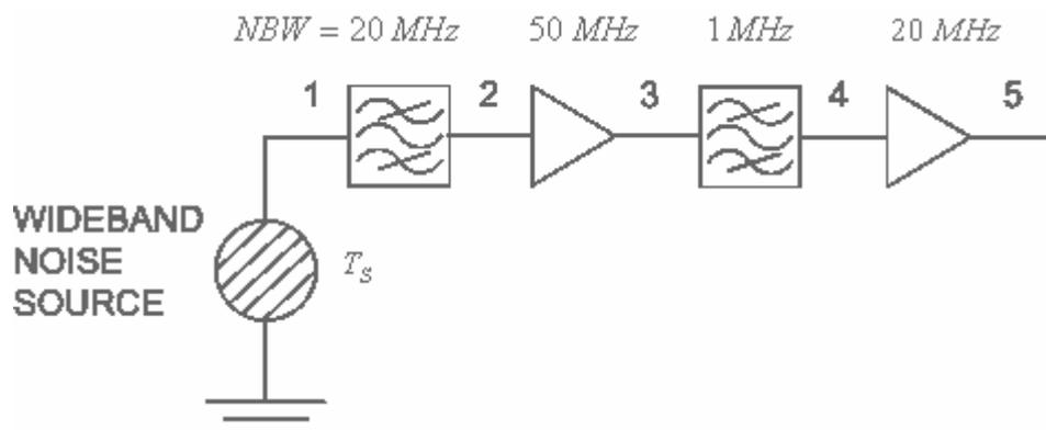
The noise bandwidths of stages 1 through to 4 are: 20 MHz, 50 MHz, 1 MHz and 20 MHz respectively. Each stage has a finite noise figure so therefore makes an individual contribution to the accumulation of noise passing through the cascade.
