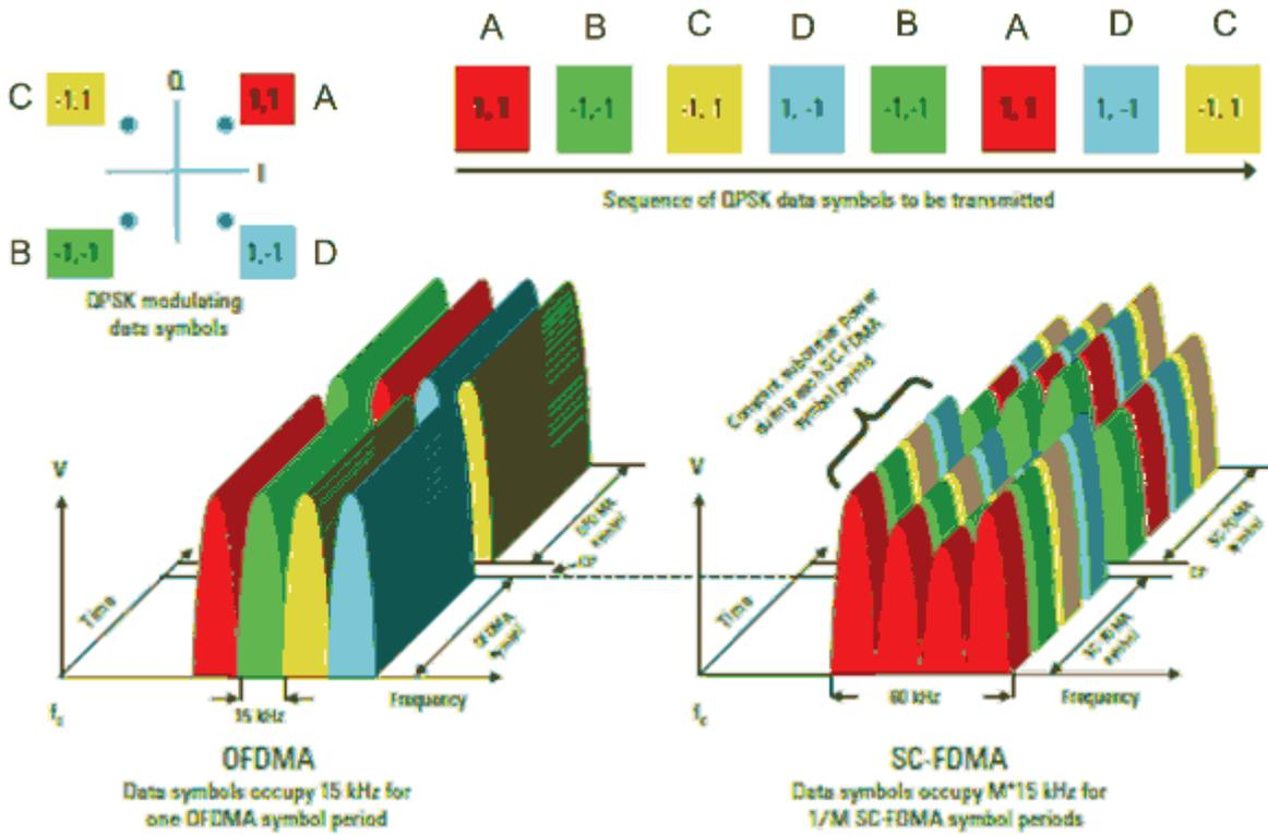
Figure 2-1 An illustration of the transmission of OFDMA and SC-FDMA in the combined voltage, frequency, time plane
