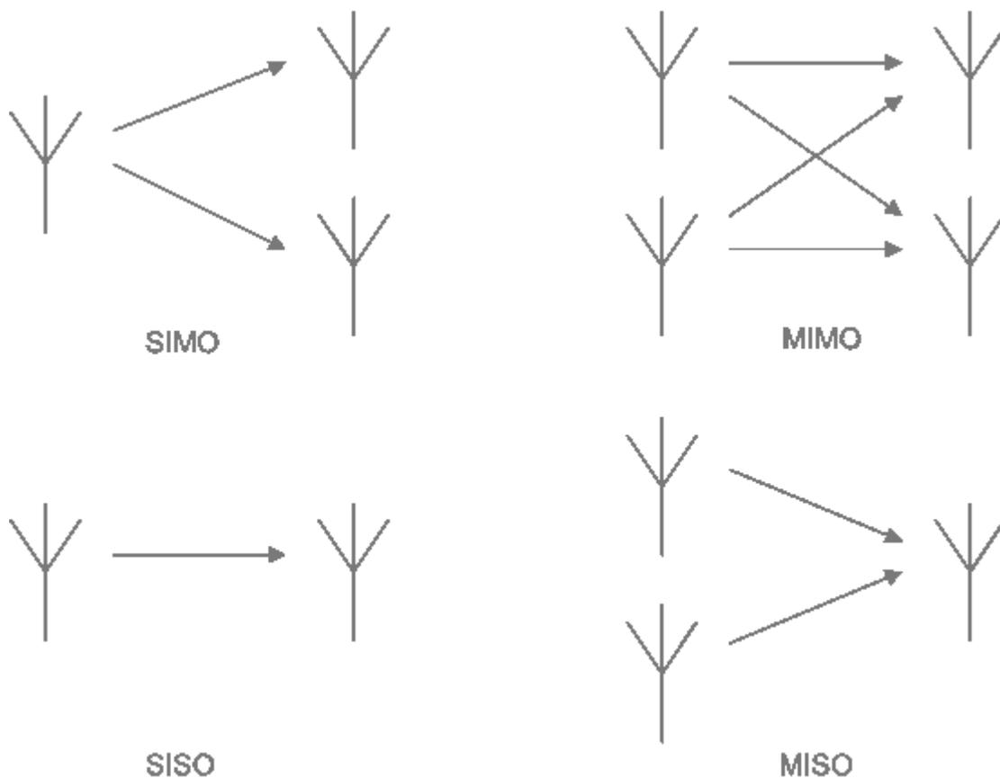
**Figure 1-1 Schematics of some multiple antenna configurations assuming a maximum of 2 at either terminal. More antennas are supported under LTE-A**
