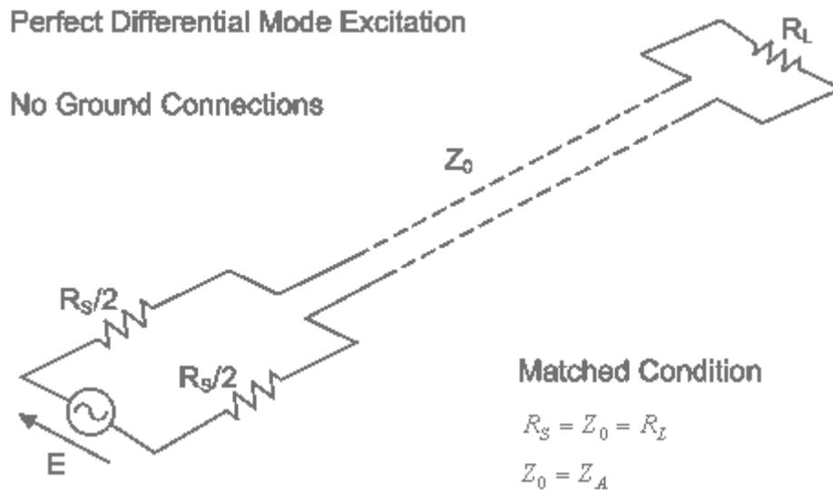
**Figure 3-2 The simplest form of differentially excited connection between a balanced source, a balanced transmission line and a balanced load**
