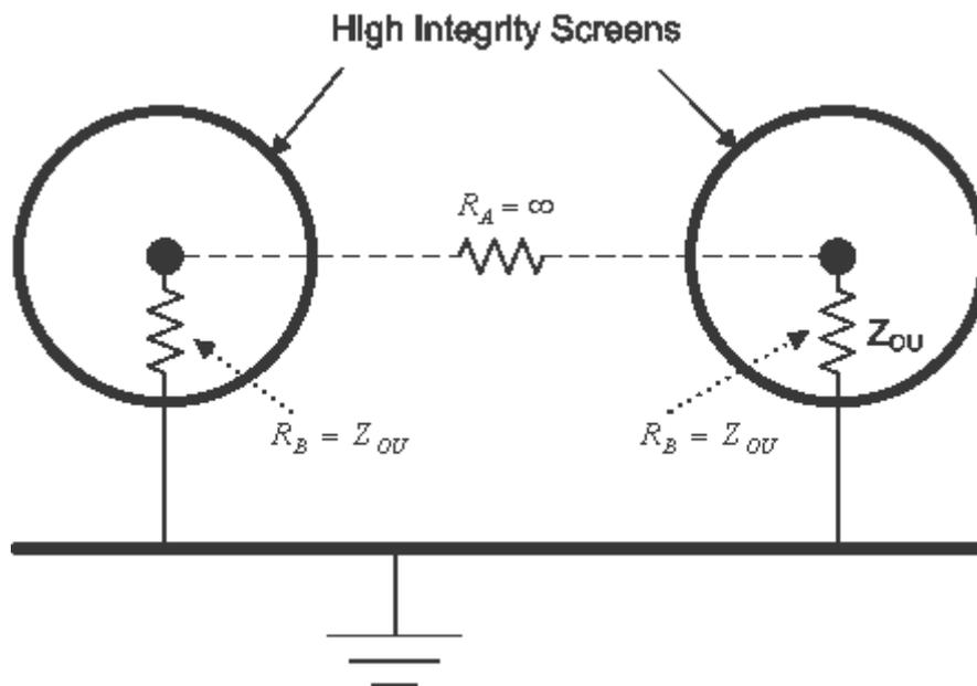
**Figure 2-10 Relating the components of characteristic impedance for the connections shown in Figure 2-8 to Figure 1-4(b)**
