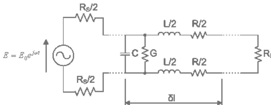
**Figure 1-3 The schematic for a two conductor lossy balanced transmission line comprising series elements of inductance and resistance with shunt elements of capacitance and conductance**
