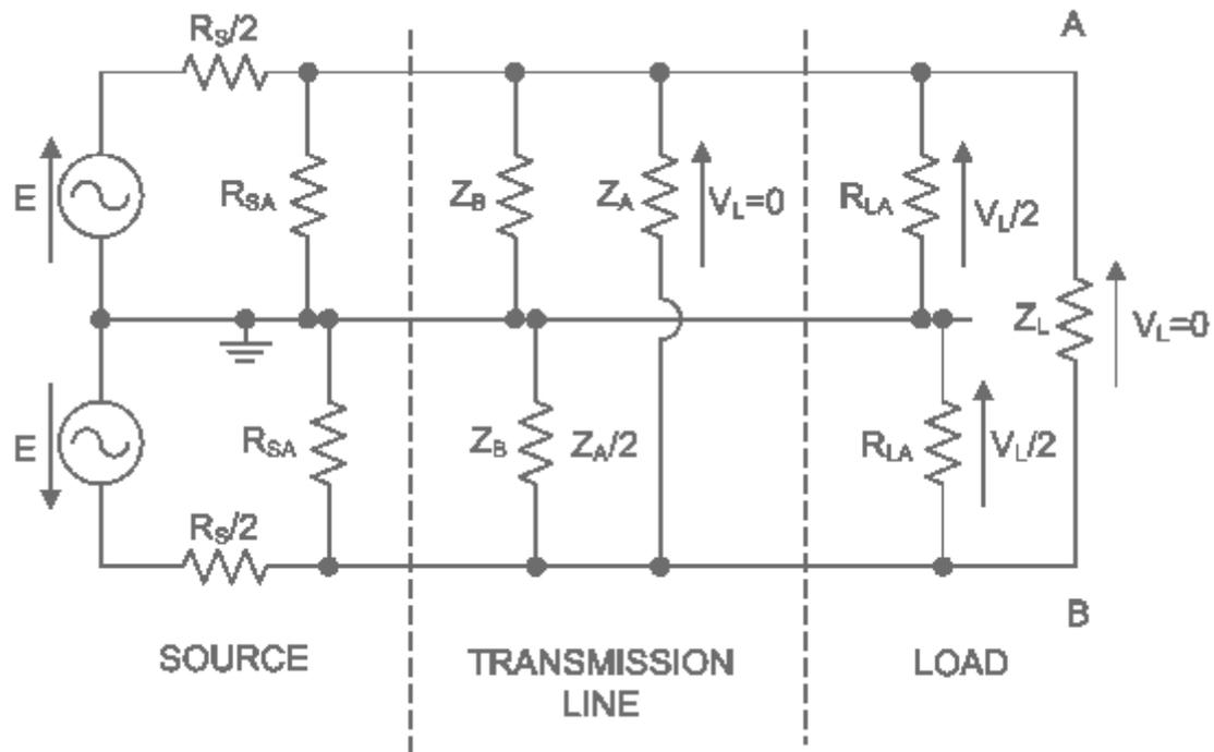
**Figure 3-10 The first stage equivalent circuit for perfectly common mode excitation**
