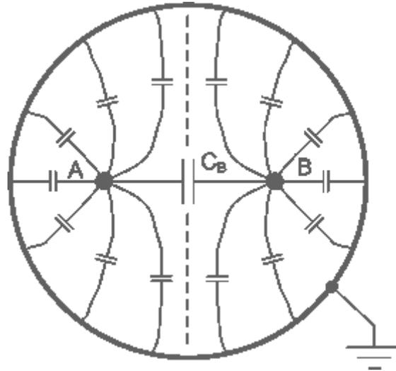
**Figure 2-4 A schematic cross section of a balanced two wire transmission line comprising wires A and B, together with a coupled cylindrical screen enclosing both and connected to ground.**
