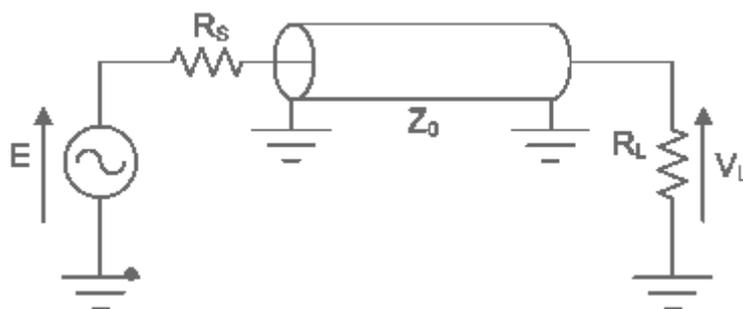
**Figure 3-1 A simple single ended (coaxial) transmission line fed by a source represented as a Thevenin equivalent circuit of source resistance  $R_S$  and feeding a load resistance  $R_L$**
