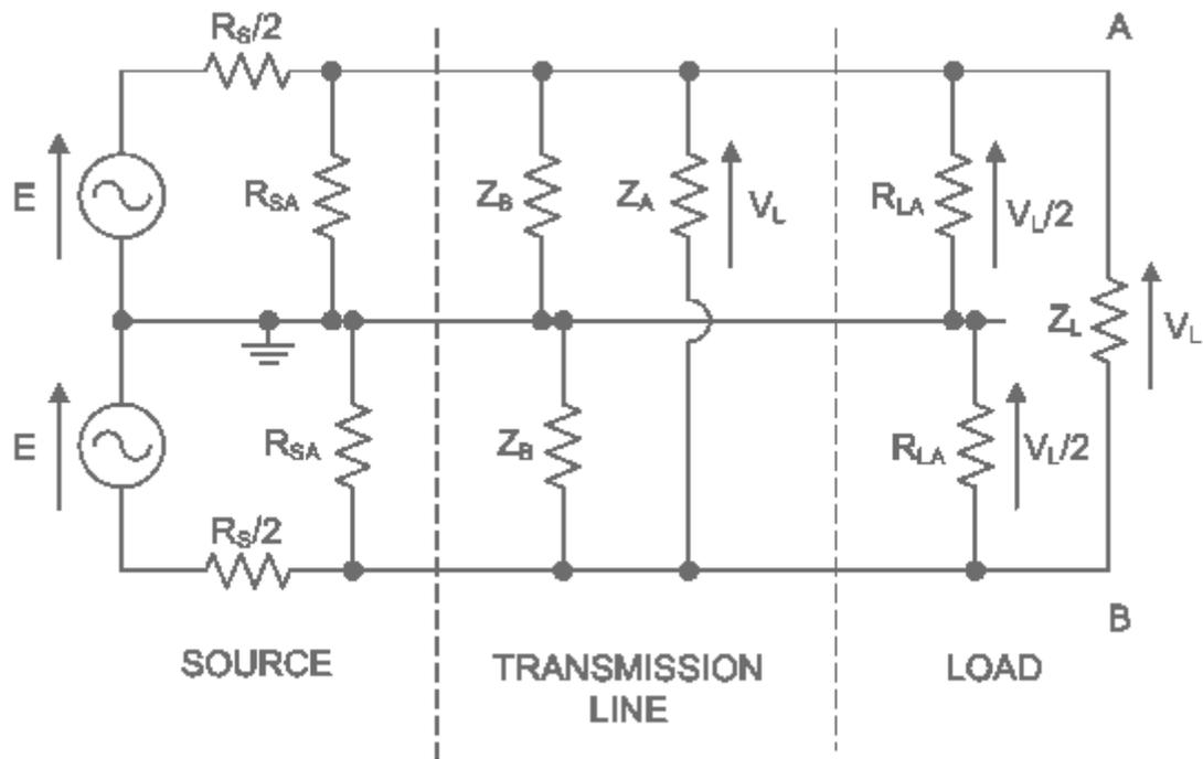
**Figure 3-5 The equivalent circuit for the perfectly differentially excited balanced circuit shown in Figure 3-4**
