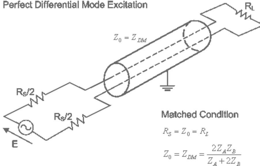
**Figure 3-3 Connection of a differentially excited balanced source to a balanced load using a screened, balanced pair transmission line**
