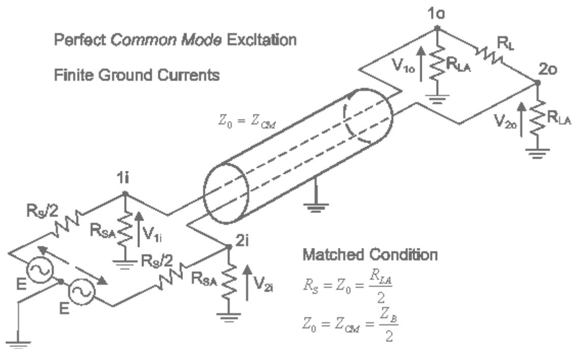
**Figure 3-9 Connection of a common mode excited balanced source to a balanced load using a screened, balanced pair transmission line. Further resistors  $R_{SA}$  and  $R_{LA}$  represent typical realistic loading conditions**
