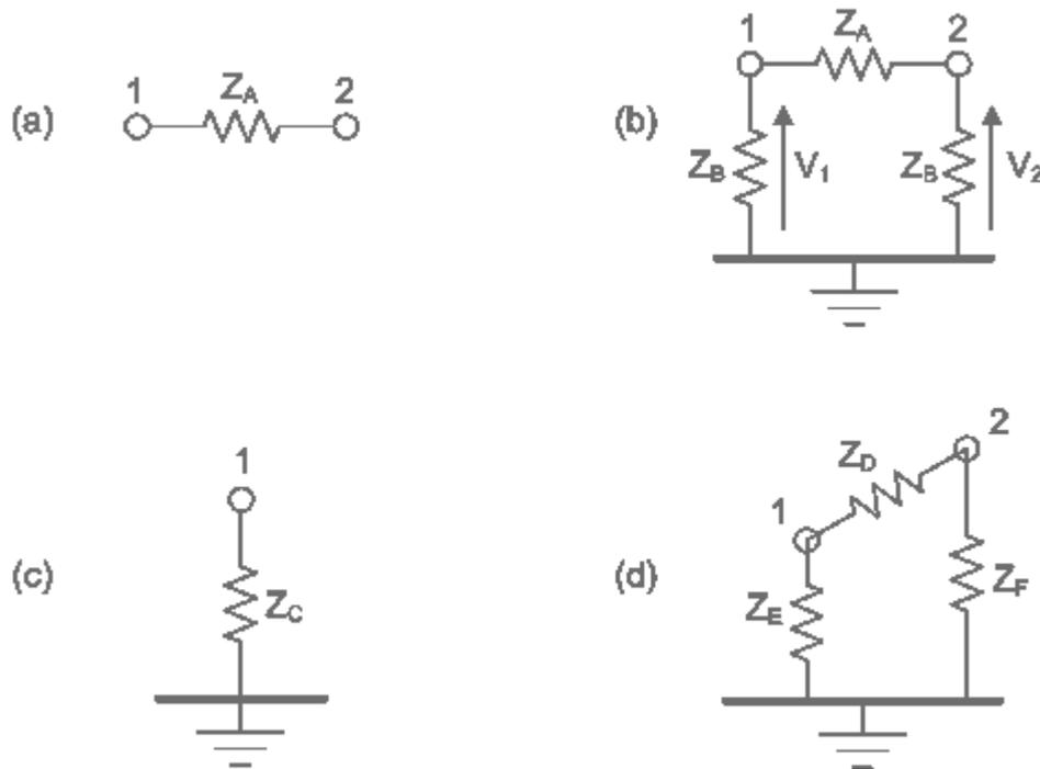
**Figure 1-4 Schematic representations of characteristic impedances for various transmission line geometries: (a) 2 wire balanced, (b) 2 wire balanced with ground, (c) single ended (unbalanced) and (d) 2 wire unbalanced (asymmetric). In each case we are considering a plane perpendicular to the direction of propagation**
