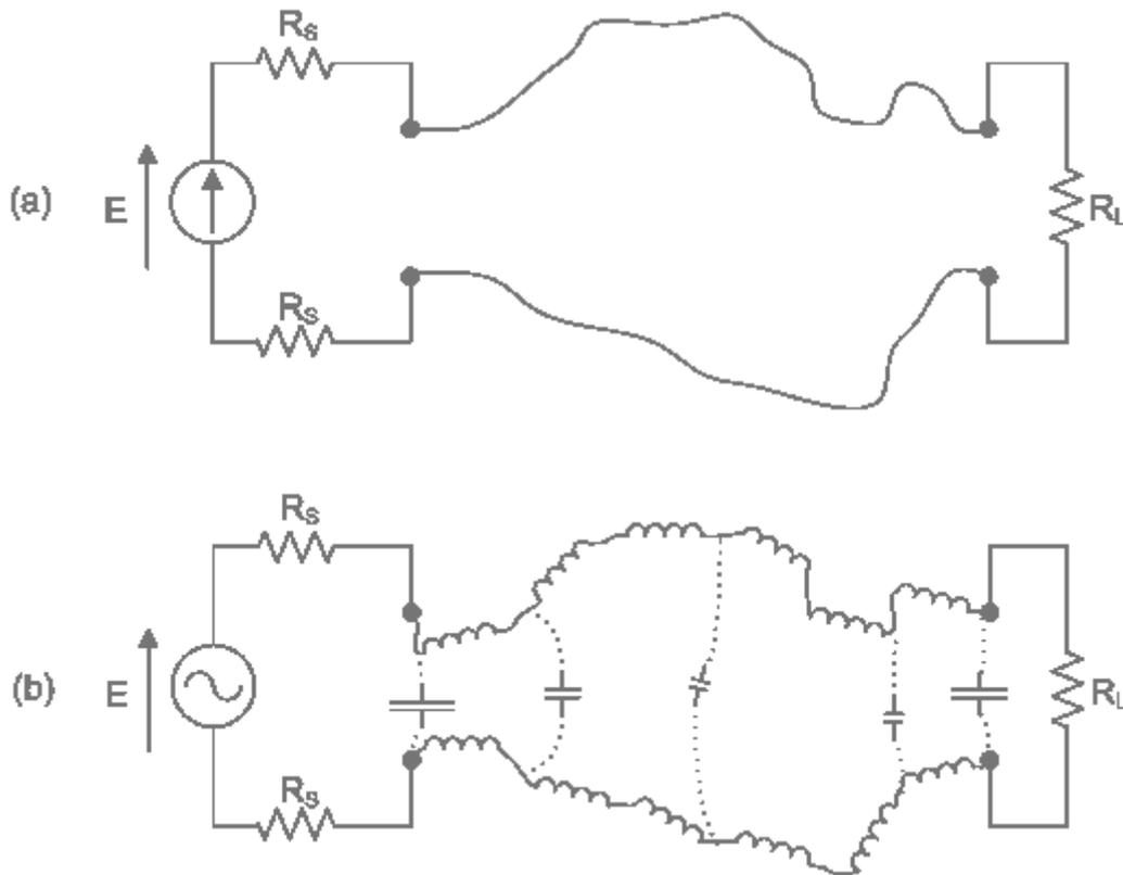
**Figure 1-1 A simple DC (a) and AC (b) circuit to transfer power from the source on the left to the load on the right. The reactive components become more influential in (b) as the frequency is increased.**
