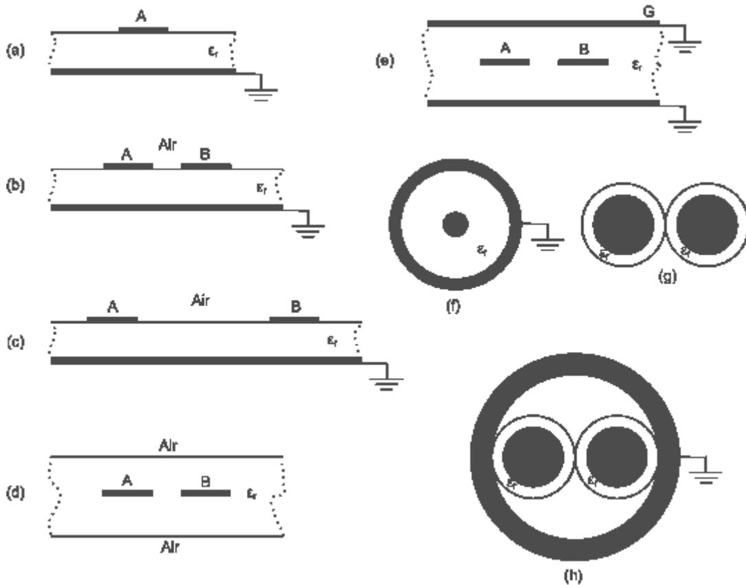
**Figure 2-2 Cross sections of various single ended and balanced transmission lines in the forms of PCBs and cables**
