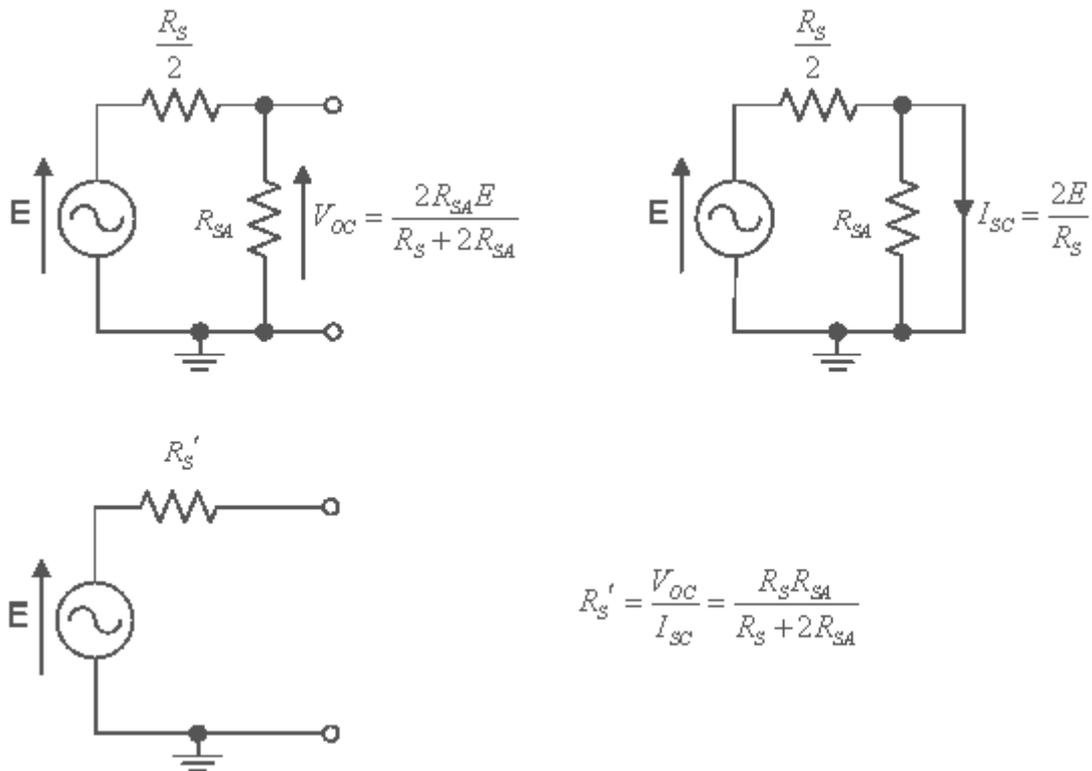
Figure 3-7 Simplification of the equivalent constant voltage source by calculating the open circuit voltage and short circuit current, hence the equivalent source resistance
