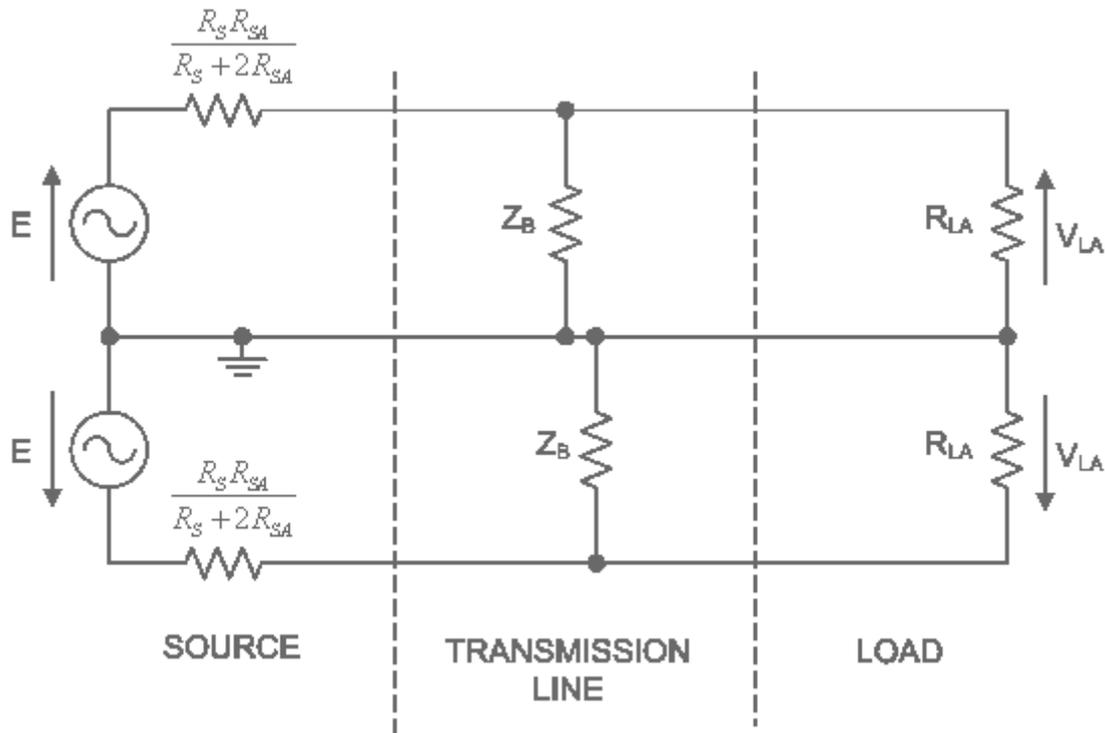
Figure 3-11 The simplified equivalent circuit for perfectly common mode excitation
