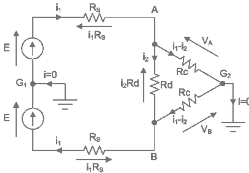
**Figure 4-2 The equivalent DC circuit schematic for perfectly differential excitation**
