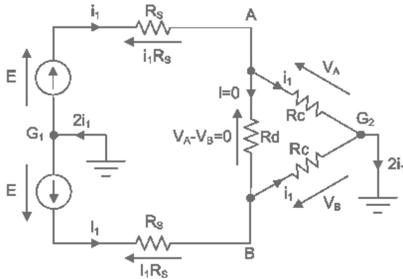
Figure 4-3 The equivalent DC circuit schematic for perfectly common mode excitation
