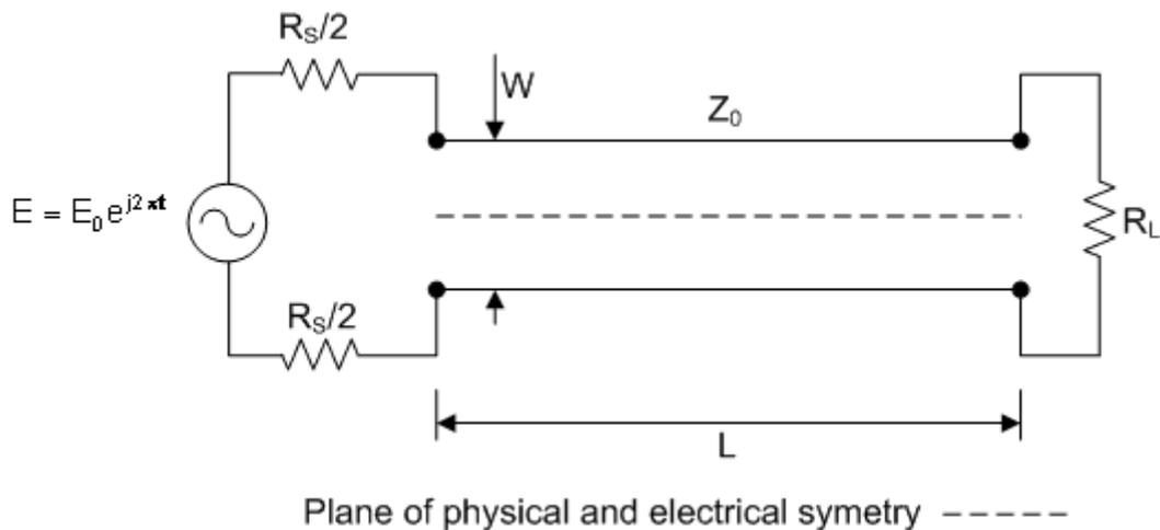
**Figure 1-2 A schematic of a simple balanced transmission line comprising two straight parallel wires of spacing  $W$  and length  $L$ : one for the ‘forward’ current and the other for the ‘return’ current**
