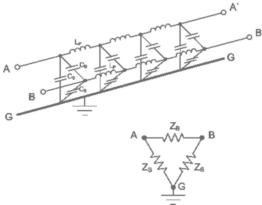
Figure 2-5 Schematic of the electrical elements of a balanced transmission line
