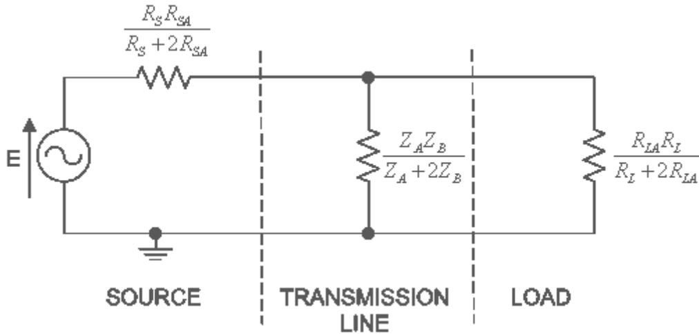
**Figure 3-8 The simplest form of the circuit shown in Figure 3-5 with perfect differential excitation**
