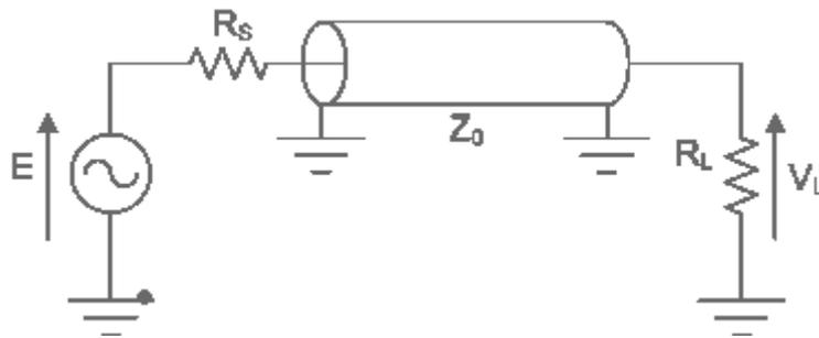
Figure 2-1 Circuit schematic of a Thevenin equivalent voltage source with source impedance  $R_s$  feeding a load of impedance  $R_L$  via coaxial transmission line with a characteristic impedance  $Z_0$
