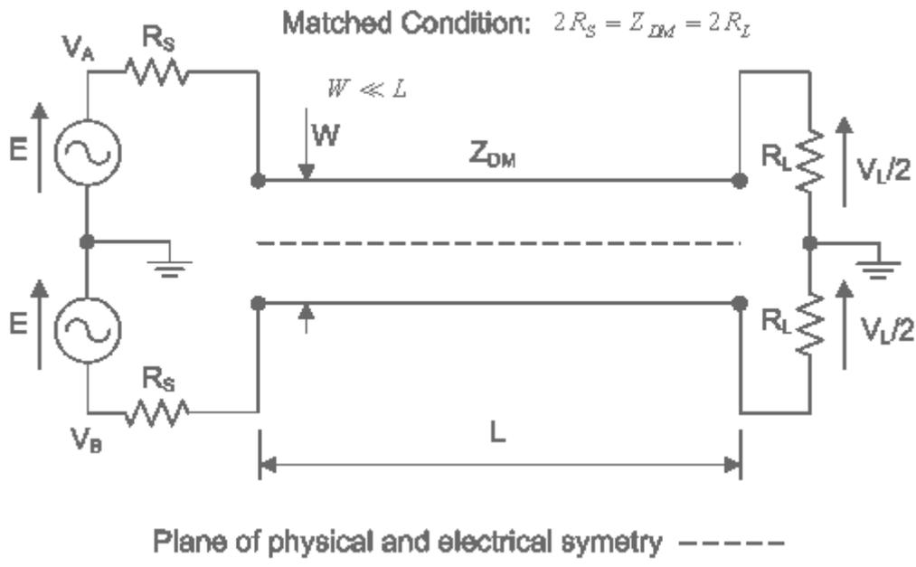
**Figure 2-7 The circuit schematic for an open wire (coupled) balanced transmission line with perfect differential excitation under which no current will flow in the ground paths.**
