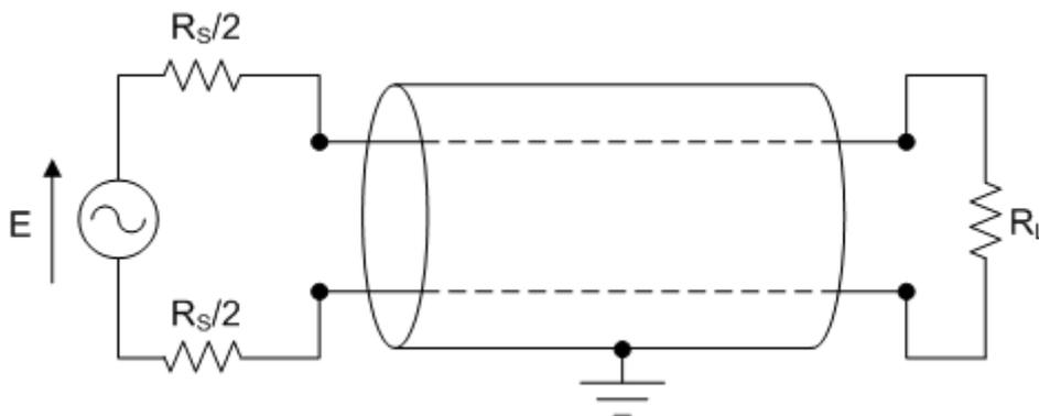
**Figure 2-3 An illustration of how a cylindrical screen, usually connected to ground, might be necessary to surround a balanced transmission line**
