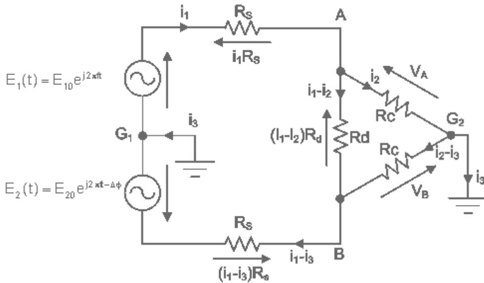
**Figure 4-1 The equivalent circuit using generic symmetric sources running at identical frequencies, arbitrary phase relationships and a symmetric load about the ground connection**
