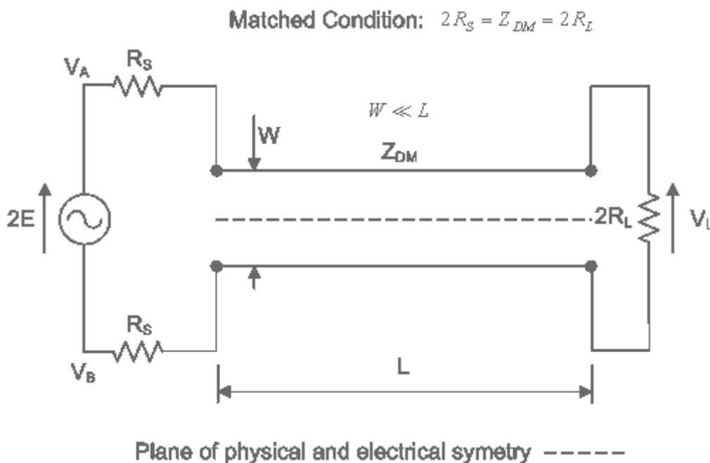
**Figure 2-6 The ideal case of an open wire (coupled, balanced) transmission line with perfect differential excitation. There are no influences from any ground connections.**
