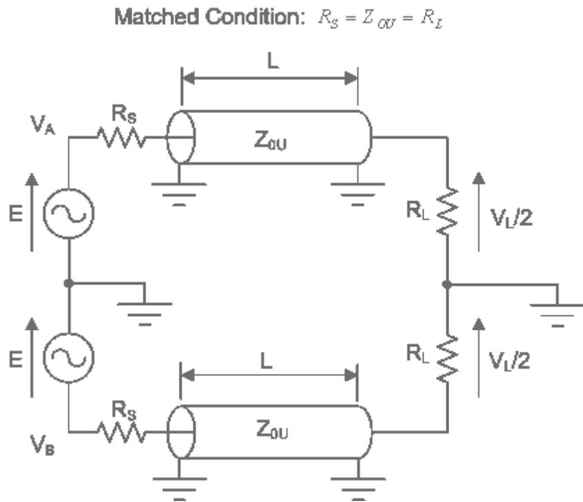
Figure 2-8 The circuit schematic for two separate coaxial lines with perfect differential mode excitation.
