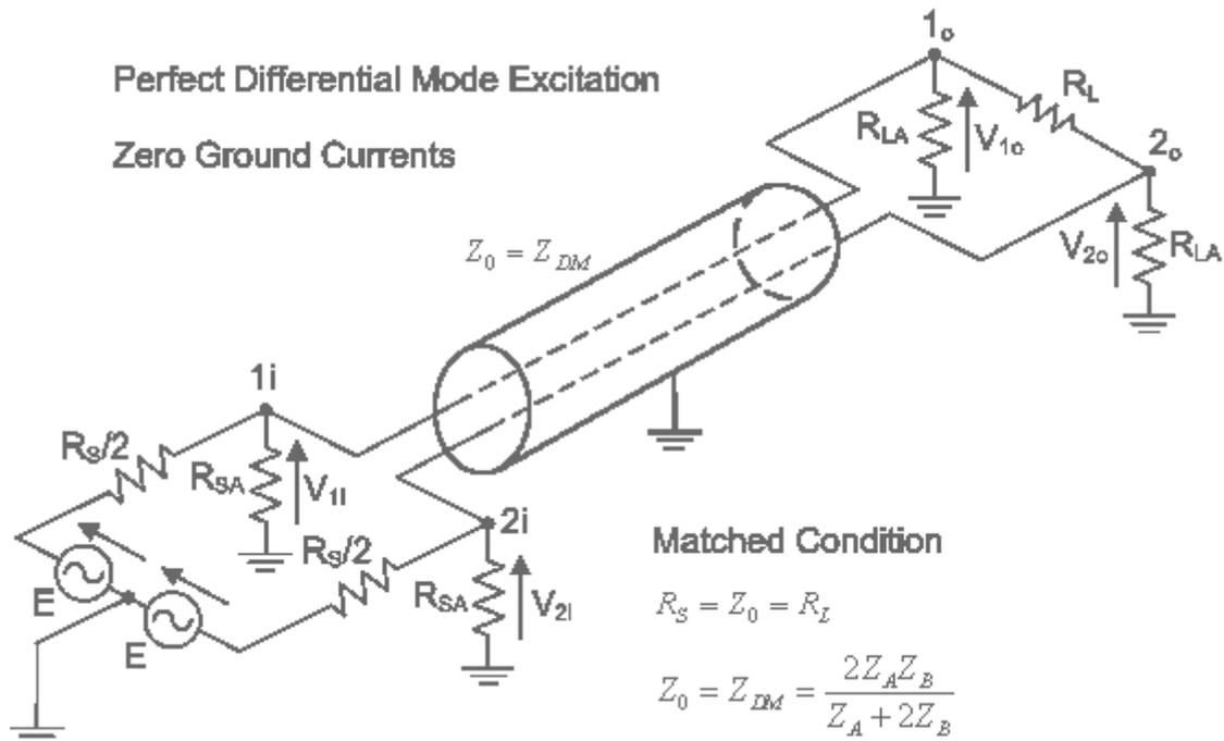
**Figure 3-4 Connection of a differentially excited balanced source to a balanced load using a screened, balanced pair transmission line. Further resistors  $R_{SA}$  and  $R_{LA}$  represent typical realistic loading conditions**
