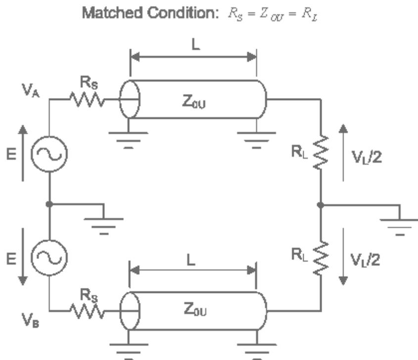
Figure 2-9 The circuit schematic for two separate coaxial lines with perfect common mode excitation.
